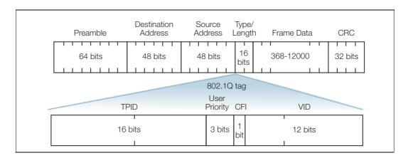
The following figure shows how the VLAN tag is inserted in the frame:
